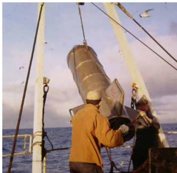
Gulf III high speed plankton sampler.
